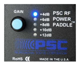
Gain settings are easily adjusted using the rotary switch. Gain setting is displayed by a lighted LED.
